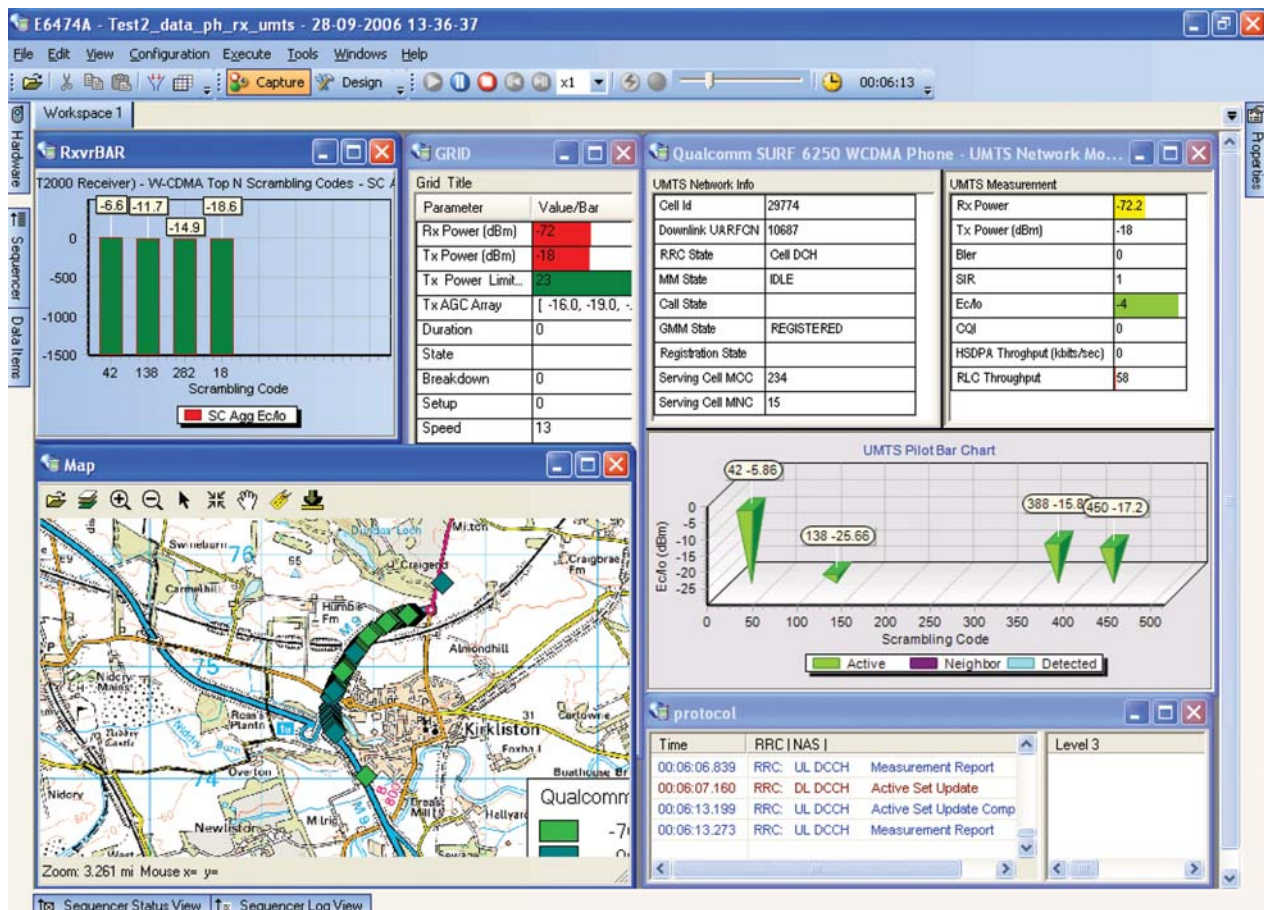
Figure 4. Maps and geolocation information can help pinpoint sources of interference.
