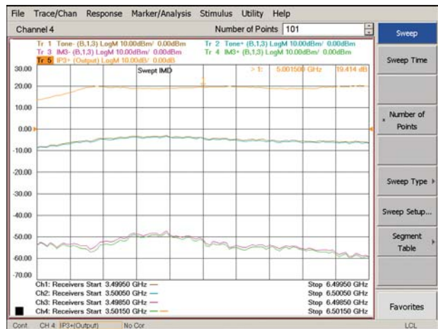
Figure 4. PNA-X example of a swept-frequency IMD measurement
