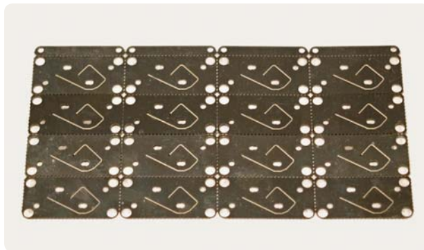
Figure 4. Photolithographic milling ensures precise channel geometry and low dead volume in capillary-flow devices.
